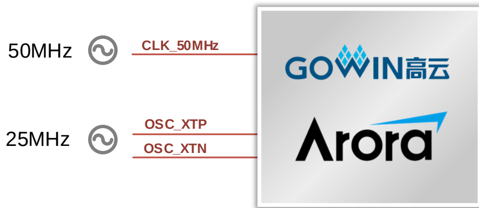
Figure 3-3 Connection Diagram of Clock
