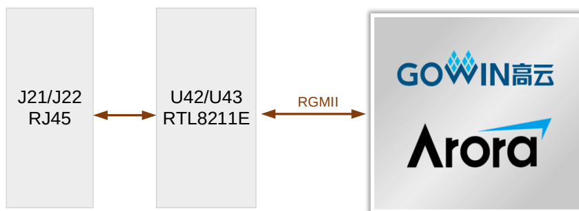
Figure 3-6 Connection Diagram of Ethernet Interface
