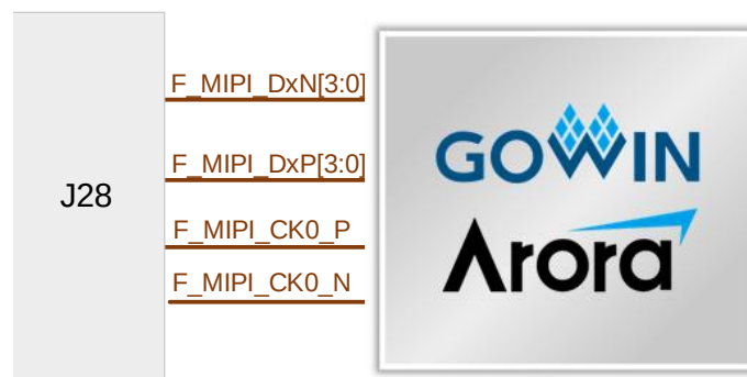
Figure 3-10 Connection Diagram of MIPI D-PHY (Soft Core) Interface
