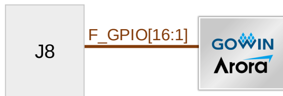
Figure 3-14 Connection Diagram of GPIO Interface
