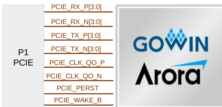
Figure 3-5 Connection Diagram of PCIe Interface
