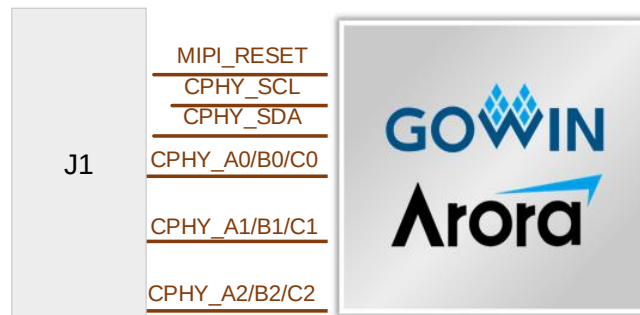
Figure 3-8 Connection Diagram of MIPI C-PHY (Hard Core) Interface
