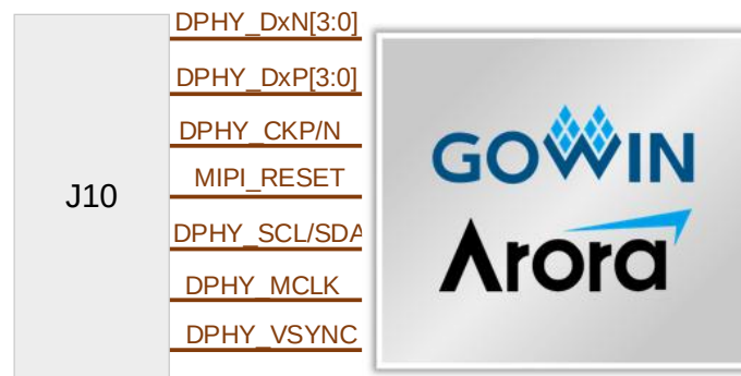
Figure 3-9 Connection Diagram of MIPI D-PHY (Hard Core) Interface
