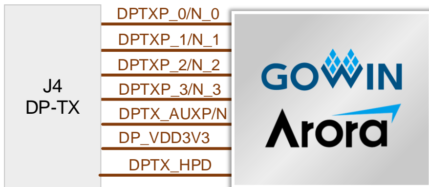
Figure 4-4 Connection Diagram of DP-TX Interface
