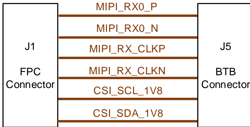
Figure 4-10 Connection Diagram of MIPI DPHY Soft Core Interface
