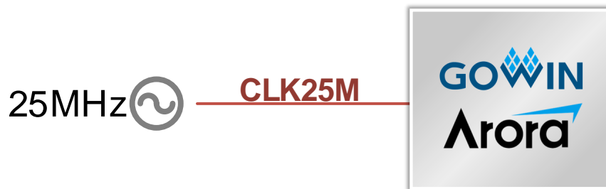
Figure 3-3 Clock Connection Diagram
