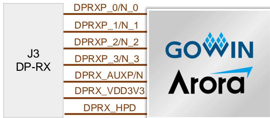
Figure 4-5 Connection Diagram of DP-RX Interface
