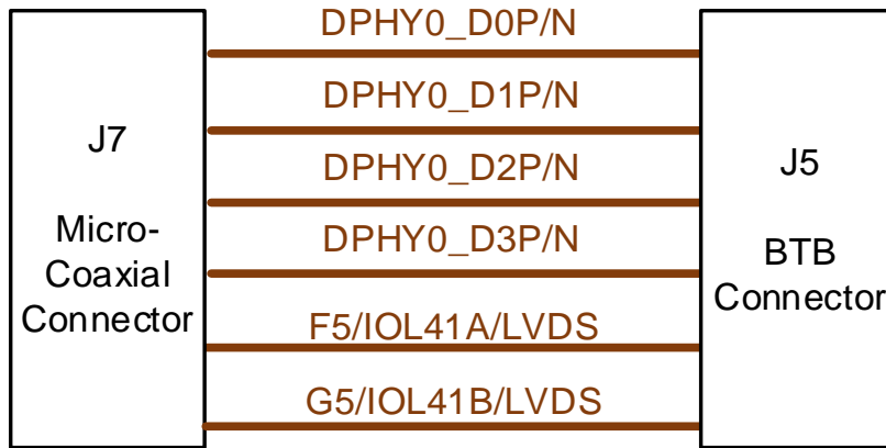
Figure 4-9 Connection Diagram of MIPI DPHY Hard Core Interface
