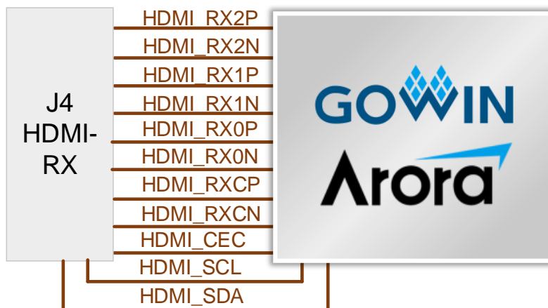
Figure 3-5 Connection Diagram of HDMI-RX Interface
