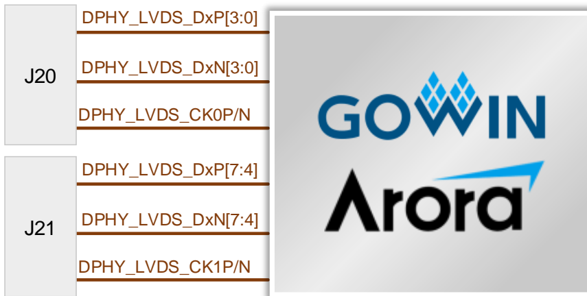
Figure 3-6 Connection Diagram of MIPI DPHY Soft Core/LVDS Interface
