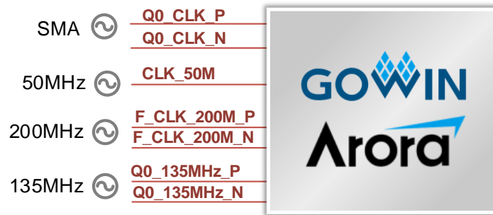
Figure 3-3 Clock Connection Diagram
