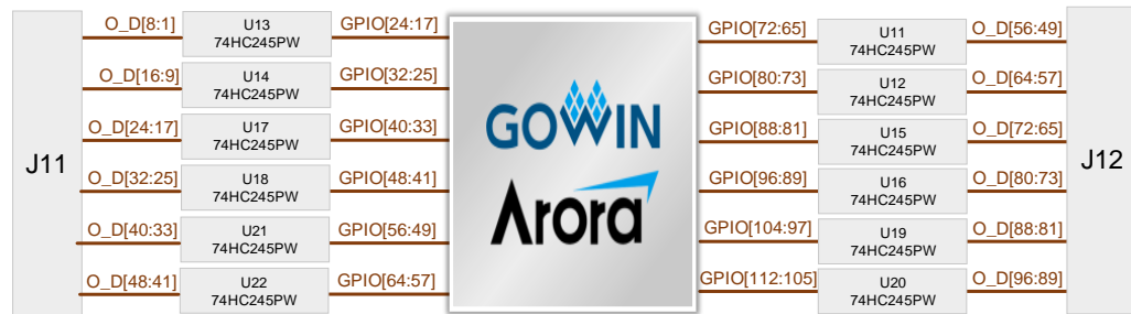
Figure 3-9 Schematic of GPIO Interface
