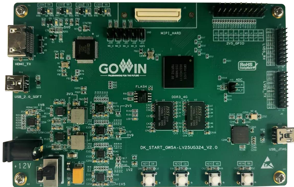
Figure 2-1 DK_START_GW5A-LV25UG324_V2.0 Development Board
