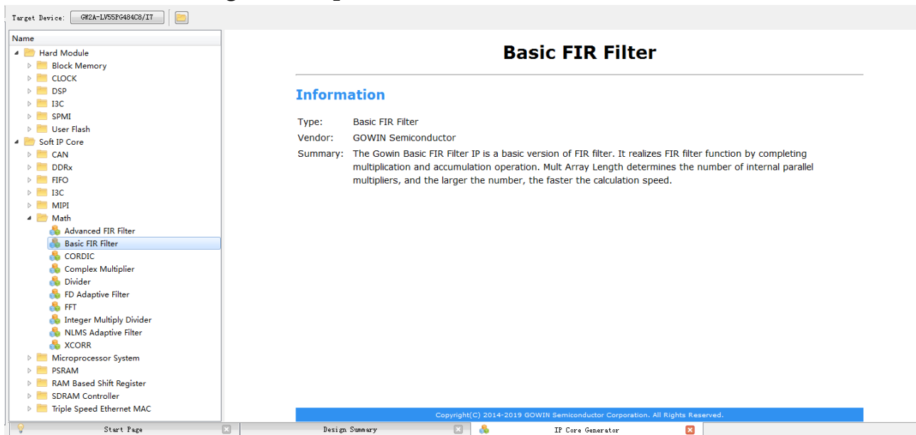
Figure 7-1 Open Basic FIR Filter IP Core
