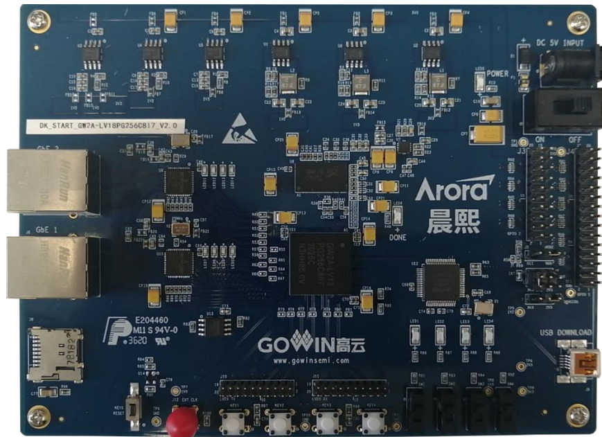
Figure 2-1 DK_START_GW2A-LV18PG256C8I7_V2.0 Development Board
